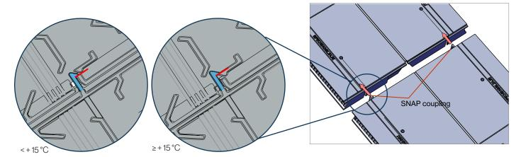
Temperature below 15 °C: attach the Airidge products together until the first notch. This leaves space for thermal expansion.
